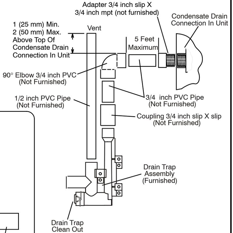
Drain Trap Assembly with 1/2 inch Piping
