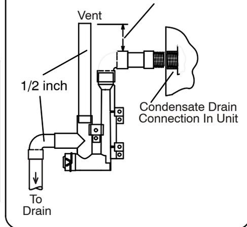
Drain Trap Assembly with 3/4 inch Piping
