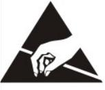
**Electrostatic discharge can affect electronic components. Take precautions to neutralize electrostatic charge by touching your hand and tools to metal prior to handling the control.**
