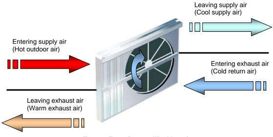
Figure 1 – Energy Recovery Wheel Operation
