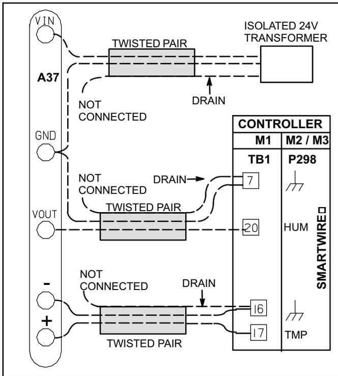
**Figure 2. Field Wiring (150' [46m] or longer runs)**
