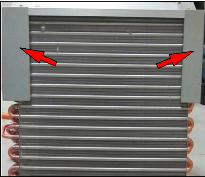
Figure 7. Reinstall the Top Cap. Brackets Must Cover the Hairpins
