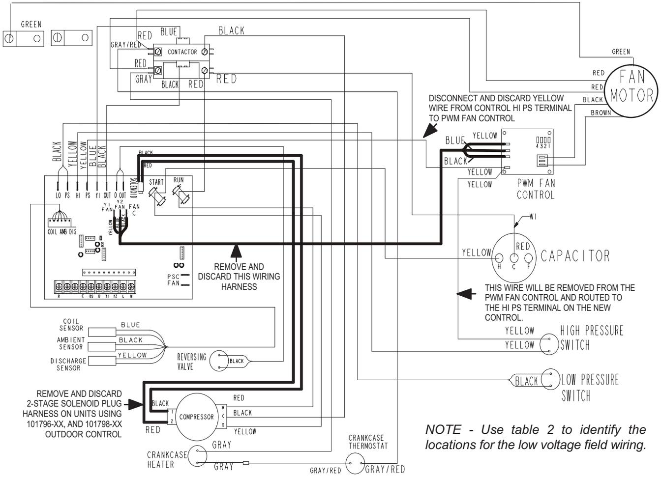
**FIGURE 5. All Units – Electronically Commutated Motor (ECM) made by EBM-PAST (Typical Original Wiring – AC or Heat Pump)**
