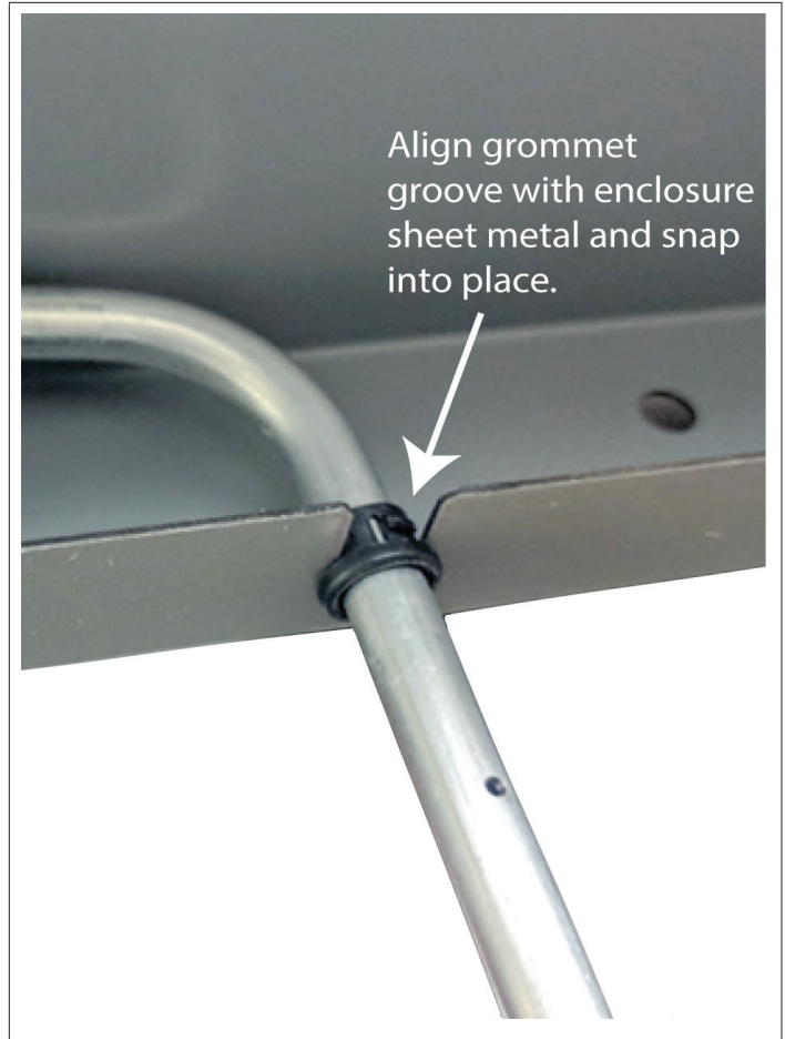
Figure 6. Snap-In Probe with Grommet
