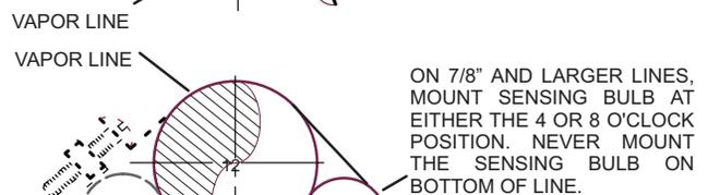
**NOTE - NEVER MOUNT THE SENSING BULB ON BOTTOM OF LINE.**
