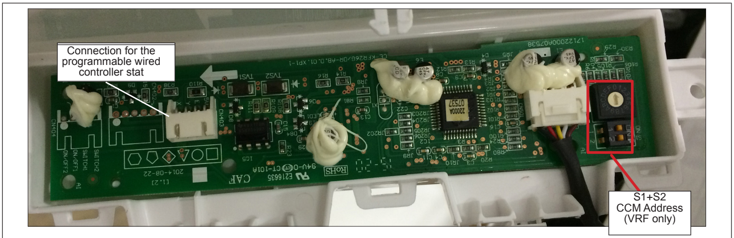
Figure 29. MWMA and MWMB Receiver Control Image (No Operation Switches on Main Control)
