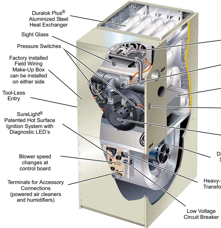
**GAS FURNACES****G51MP****ELITE® SERIES****Multi-Position - Direct Vent/Non-Direct Vent****AFUE - up to 92.5%****Input - 44,000 to 132,000 Btuh****Nominal Add-on Cooling - 2 to 5 tons**Toronto
