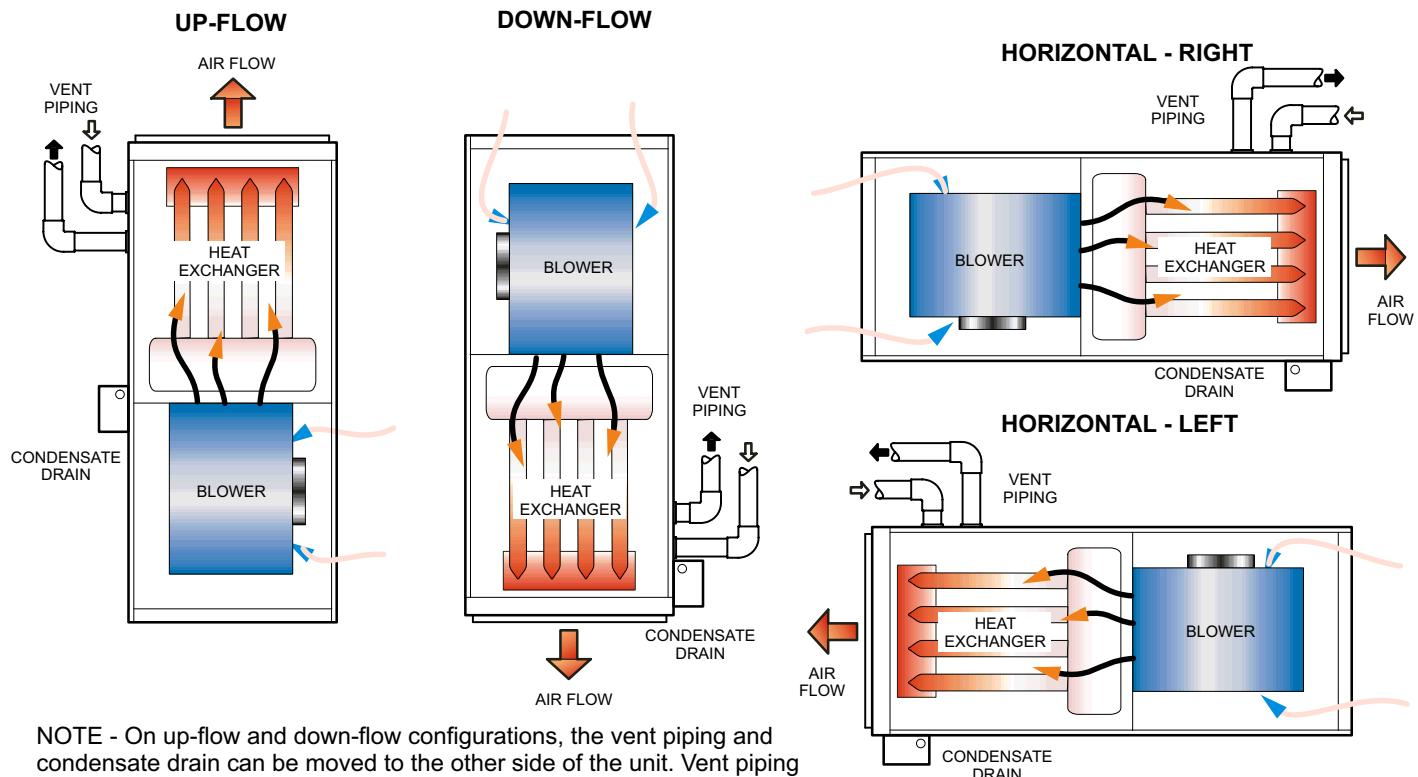
NOTE - On up-flow and down-flow configurations, the vent piping and condensate drain can be moved to the other side of the unit. Vent piping and drain must be installed on the same side of the unit with each other unless optional Condensate Trap Alternate Location Kit (up-flow only) is used. On horizontal installations the drain must be located at the bottom and the vent piping at the top.
