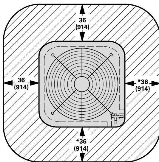
NOTE—48 in. (1219 mm) clearance required on top of unit.
