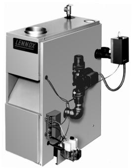
**Burners** — Each burner has four rows of continuous ports which result in quiet and clean combustion. Cast iron burners are furnished on boilers equipped for natural gas operation. Burners are constructed of stainless steel for LPG/Propane models.
