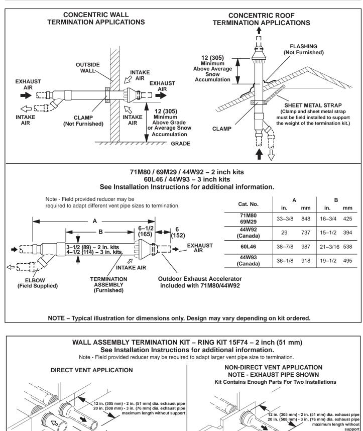
NOTE – 12 in. (305 mm) minimum height above average snow accumulation (from bottom of vent pipe).
