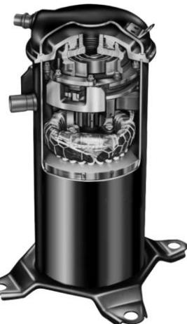
Compressor consists of two involute spiral scrolls matched together to generate a series of crescent shaped gas pockets between them.
