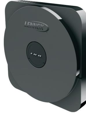
Secure wall mount for the High Definition Color Display. Sends data between the Display/Mag-Mount and the Smart Hub Controller through 4-wire, 18-gauge standard thermostat wiring.
