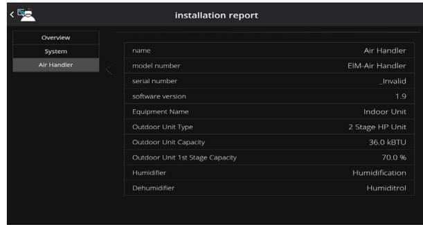
Displays various parameters and settings for the system, system and indoor equipment at the time of installation.
