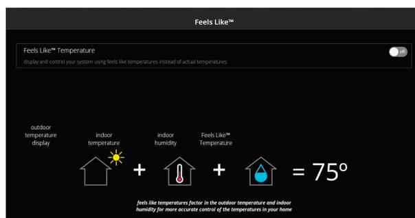
Accurately controls temperature in the home by determining the "feels like" temperature based on outdoor temperature, indoor temperature plus indoor relative humidity.
