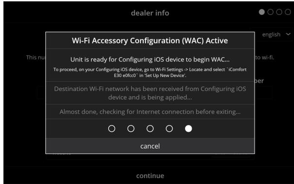
After power is applied to the thermostat for the first time, it displays the iComfort® “splash screen” (see page 21), then the Wi-Fi Accessory Configuration (**WAC**) Active screen for configuring the IOS device will appear on top of the dealer info setup screen.
