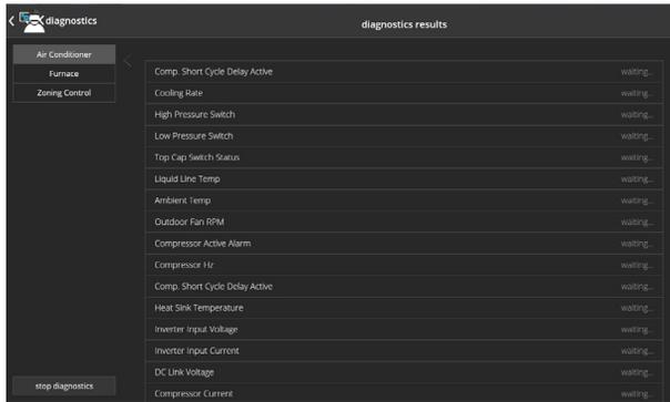
Allows the installer to test indoor unit for a variety of conditions.
