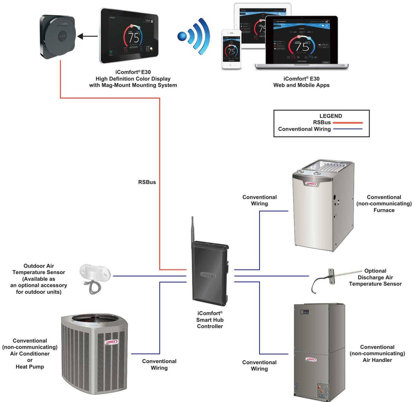
**NOTE** - The Lennox iComfort® E30 smart thermostat will also work with most conventional (non-communicating) 24VAC furnaces, air conditioners, air handlers and heat pumps (up to 3 stages of heat and 2 stages of cooling).
