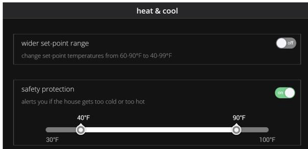
Adjustments for heating and cooling setpoints, auxiliary heat, safety protection and other settings.
