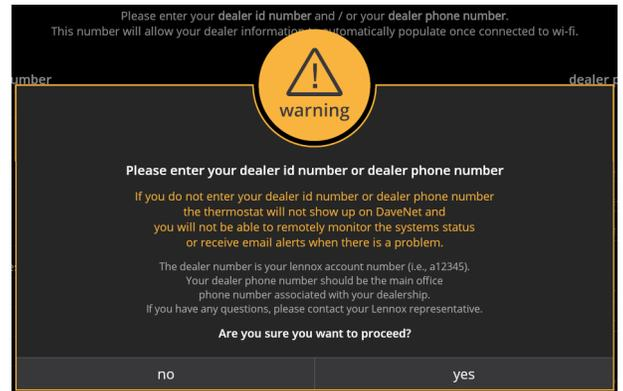
**NOTE** - If the installer does not input a dealer number or phone number, a warning screen pops up warning that this thermostat will not be visible on the LennoxPros® website and that the dealer will not be able to remotely monitor this system or receive email alerts.
