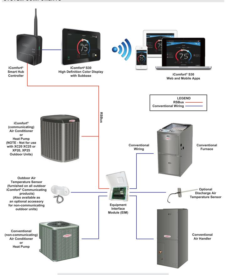
**ATTENTION** - The Lennox iComfort® Communicating Thermostat with Equipment Interface Module (EIM) will work with most 24VAC furnaces, air conditioners, air handlers and heat pumps (up to 3 stages of heat and 2 stages of cooling), **EXCEPT** it will NOT work with any brand of <u>communicating</u> HVAC equipment other than LENNOX®.
