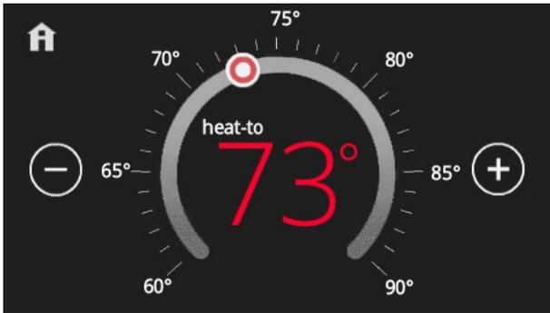
On the Home Screen, touching the heat setpoint indicators on the round temperature band, or touching the **heat-to** button displays the heat menu screen.
