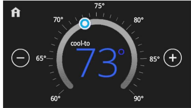
On the Home Screen, touching the cool setpoint indicators on the round temperature band, or touching the **cool-to** button displays the cool menu screen.
