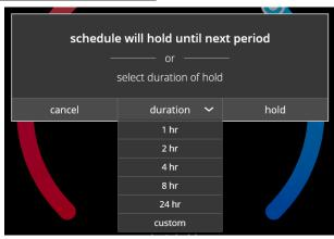
The **schedule hold** screen is displayed after changing the temperatures on the heating or cooling screens while a schedule is running. Preset 1, 2, 8, 24 hours or custom setting (using the Time Tool) sets and hold the temperature for a preset or custom time period until the next time period setting. **Cancel schedule hold** button on Home Screen cancels the held setting.
