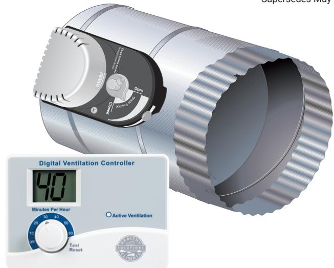
extreme hot, cold or humid air from being used to ventilate the house. The Digital Ventilation Controller prevents ventilation operation when indoor relative humidity is above 55% and the outside temperature is above 50°F to prevent excess indoor humidity levels.
