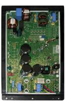
Power Factor Correction (PFC) circuit monitors the DC bus for high, low and abnormal voltage conditions to protect the compressor.
