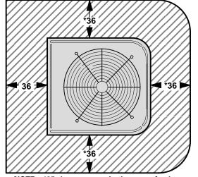
NOTE-48" clearance required on top of unit. \*NOTE-One side of coil may be 12 inches.
