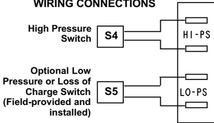
**NOTE - Jumper must be installed across HI-PS and LO-PS terminals when pressure switches are not used.**
