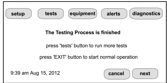
Figure 20. Testing Finished Screen
