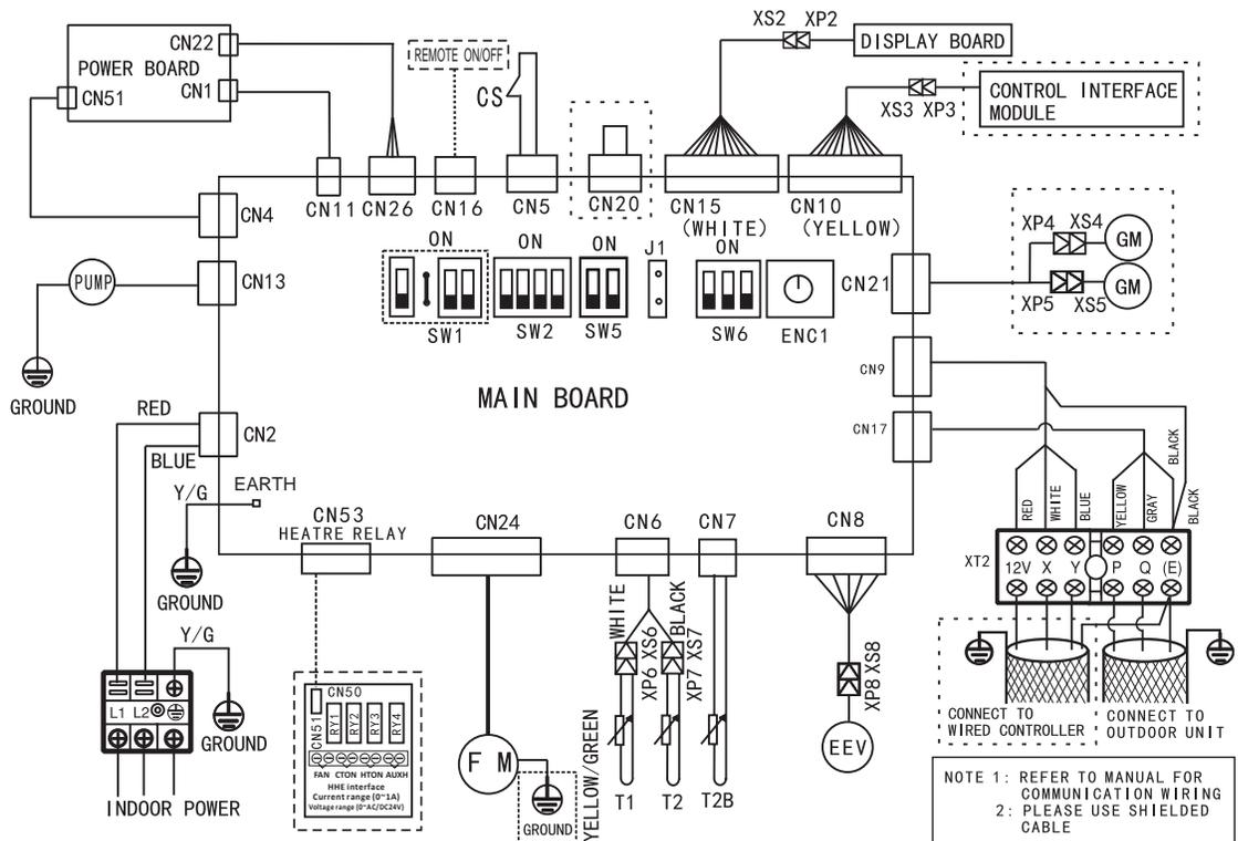
Typical wiring diagram. Refer to wiring diagram on the unit for actual wiring.
