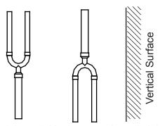
Indoor unit branch kits have graduated piping diameters. The piping can be cut to suit the installation needs. Use a pipe cutter designed for refrigeration tubing. Discard unused pipe.
