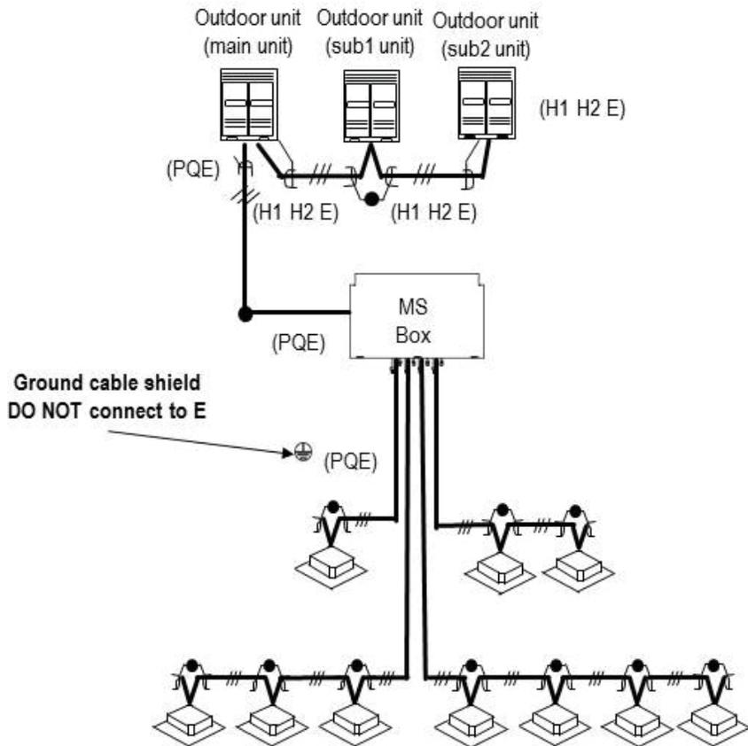
Install a terminating resistor at the last indoor unit (terminals P and Q) of the daisy chain.
