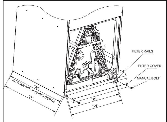
Figure 8. Air Filter Location
