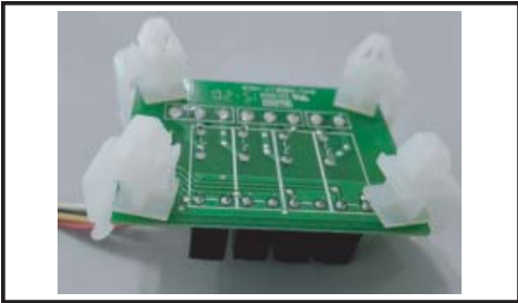
Figure 2. Mounting Feet Installed
