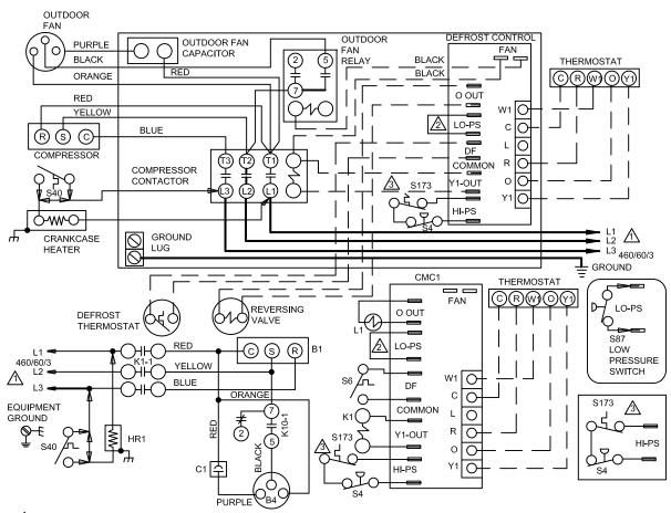
NOTE-FOR USE WITH COPPER CONDUCTORS ONLY. REFER TO UNIT RATING PLATE FOR MINIMUM CIRCUIT AMPACITY AND MAXIMUM OVERCURRENT PROTECTION SIZE
