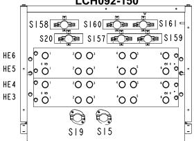
Note - Electric heat with the most components is shown. Components and location will vary by electric heat size.
