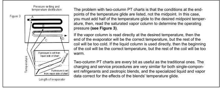
Just remember to keep track of the phase of the blend at the point you are interested: saturated vapor uses the vapor (dew point) column and saturated liquid uses the liquid (bubble point) column.
