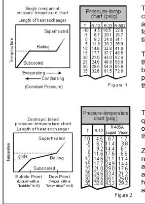
Traditional PT charts list the saturated refrigerant pressure, in psig, with a column for temperature down the left side. Single-component refrigerants and boil and condense at one temperature for a given pressure. Therefore, only one column is needed to show the pressure-temperature relationship for any phase-change process in a system (see Figure 1).
