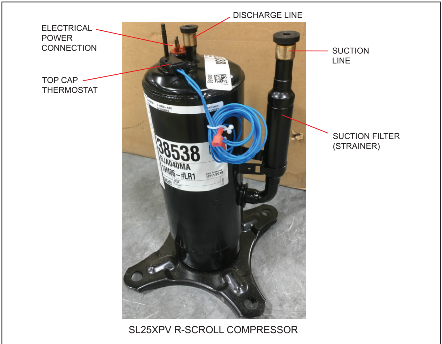
FIGURE 39. SL25XPV R-Scroll Compressor Detail
