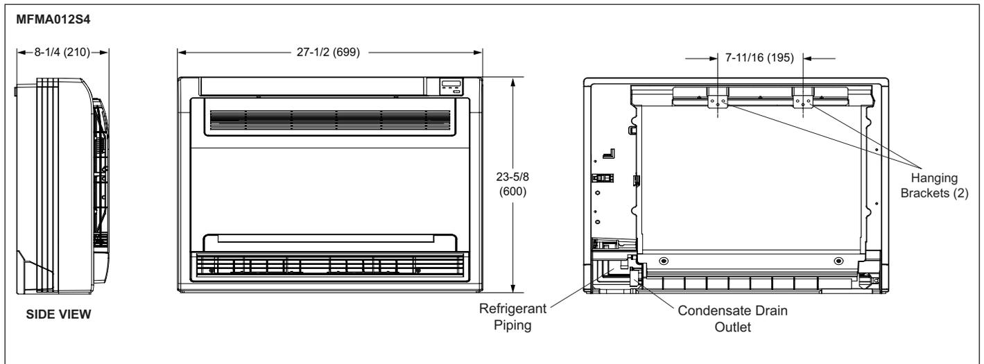
Figure 15. MFMA Indoor Unit Dimensions - Inches (mm)
