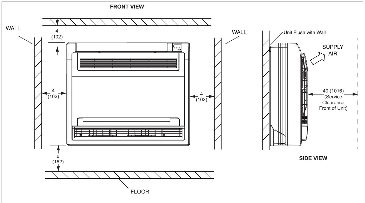
Figure 16. Indoor Unit Clearances - Inches (mm)
