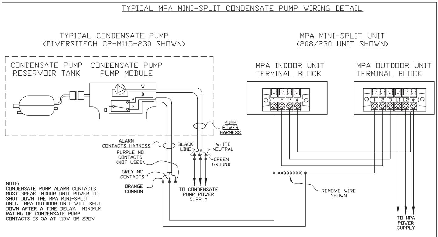
**Figure 34. MPC Condensate Pump Powered by Separate Source Wiring Diagram**
