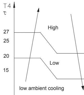
Outdoor fan speed control logical (low ambient cooling).
