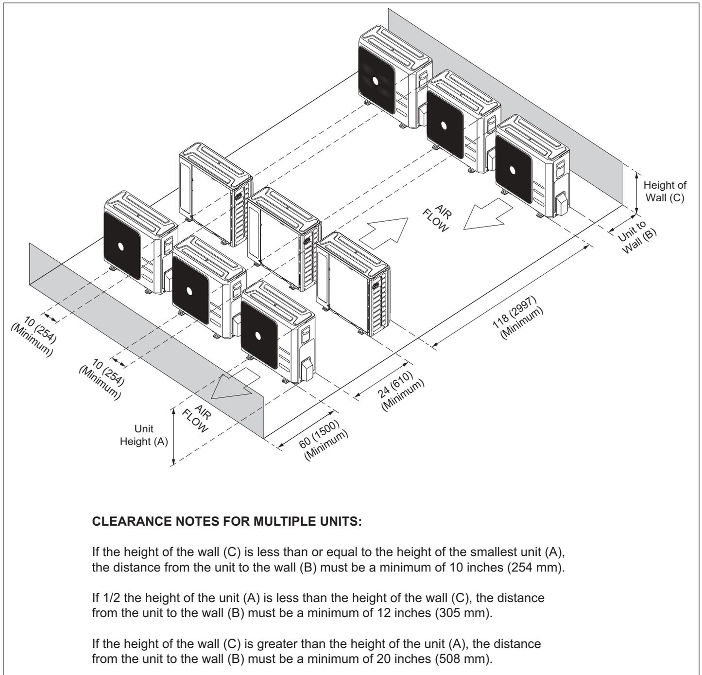
**Figure 29. Multiple Outdoor Unit Clearances - Inches (mm)**
