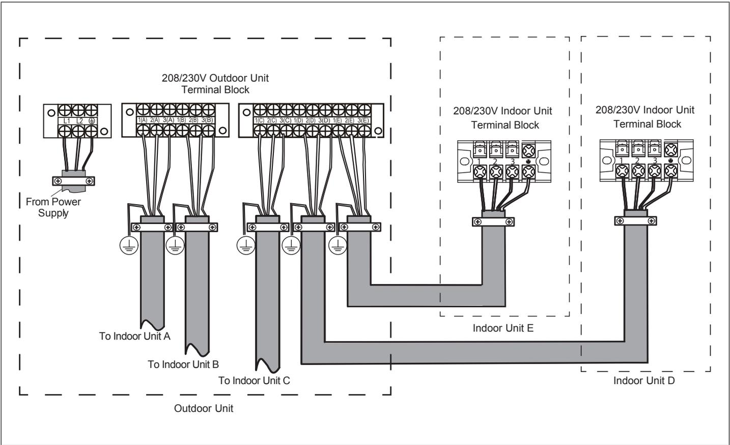
**Figure 19. Multi-Zone Wiring**
