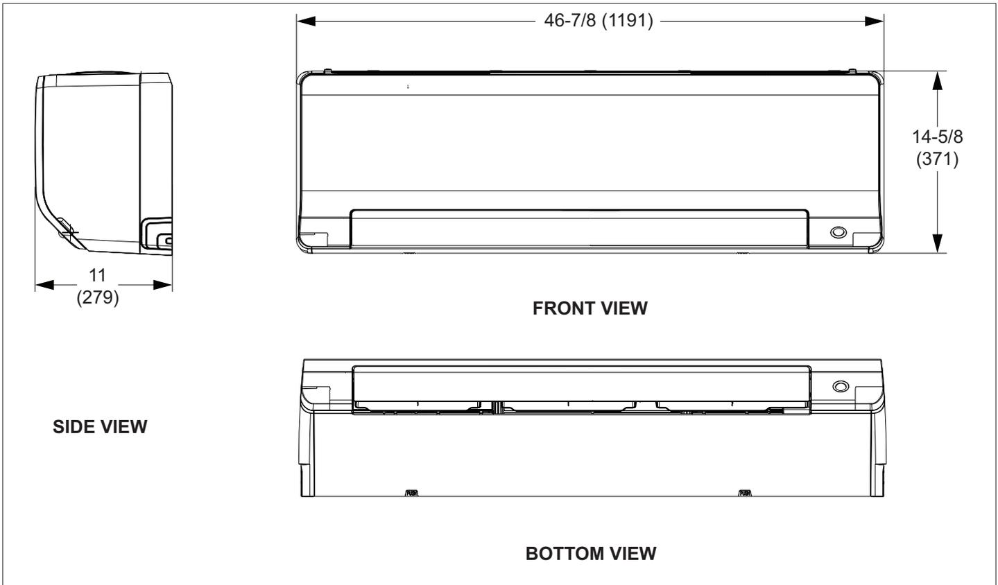
Figure 11. 3WMC036S4 Indoor Unit Dimensions - Inches (mm)
