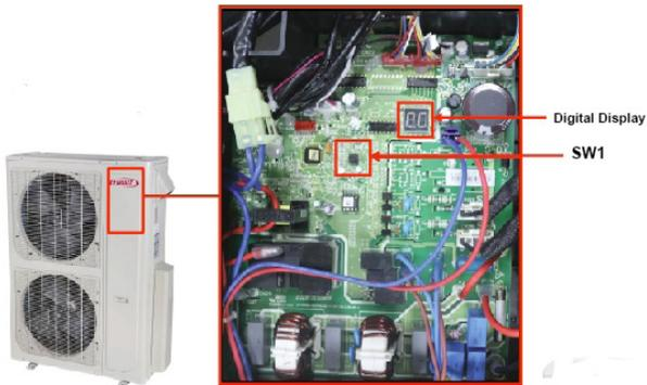
Figure 37. Typical Location of LEDs and SW1 - 36K and 48K Multi-Zone Outdoor Units
