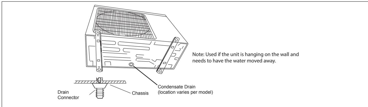
**Figure 32. Condensate Drainage Requirement**
