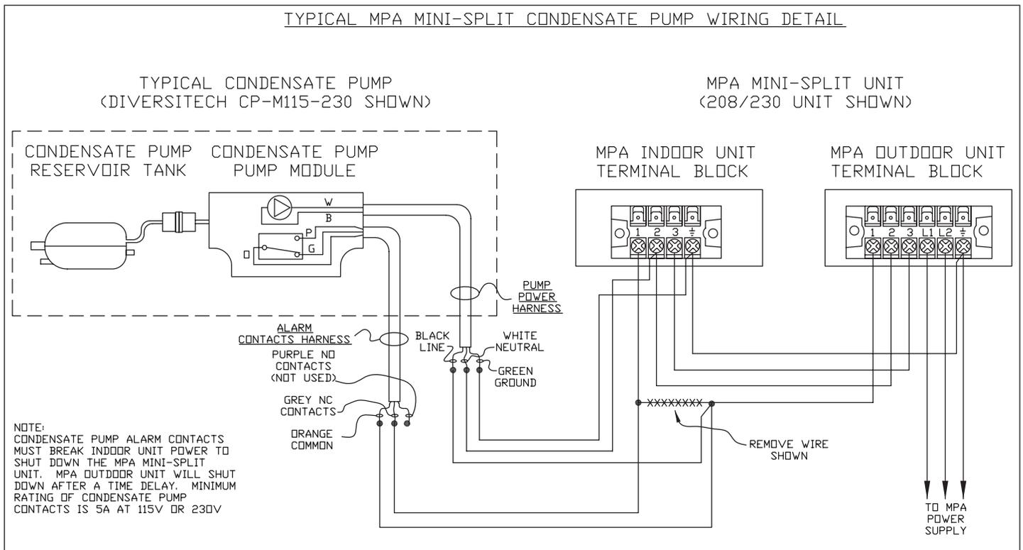
**Figure 33. MPC Condensate Pump Powered by MPA Wiring Diagram**
