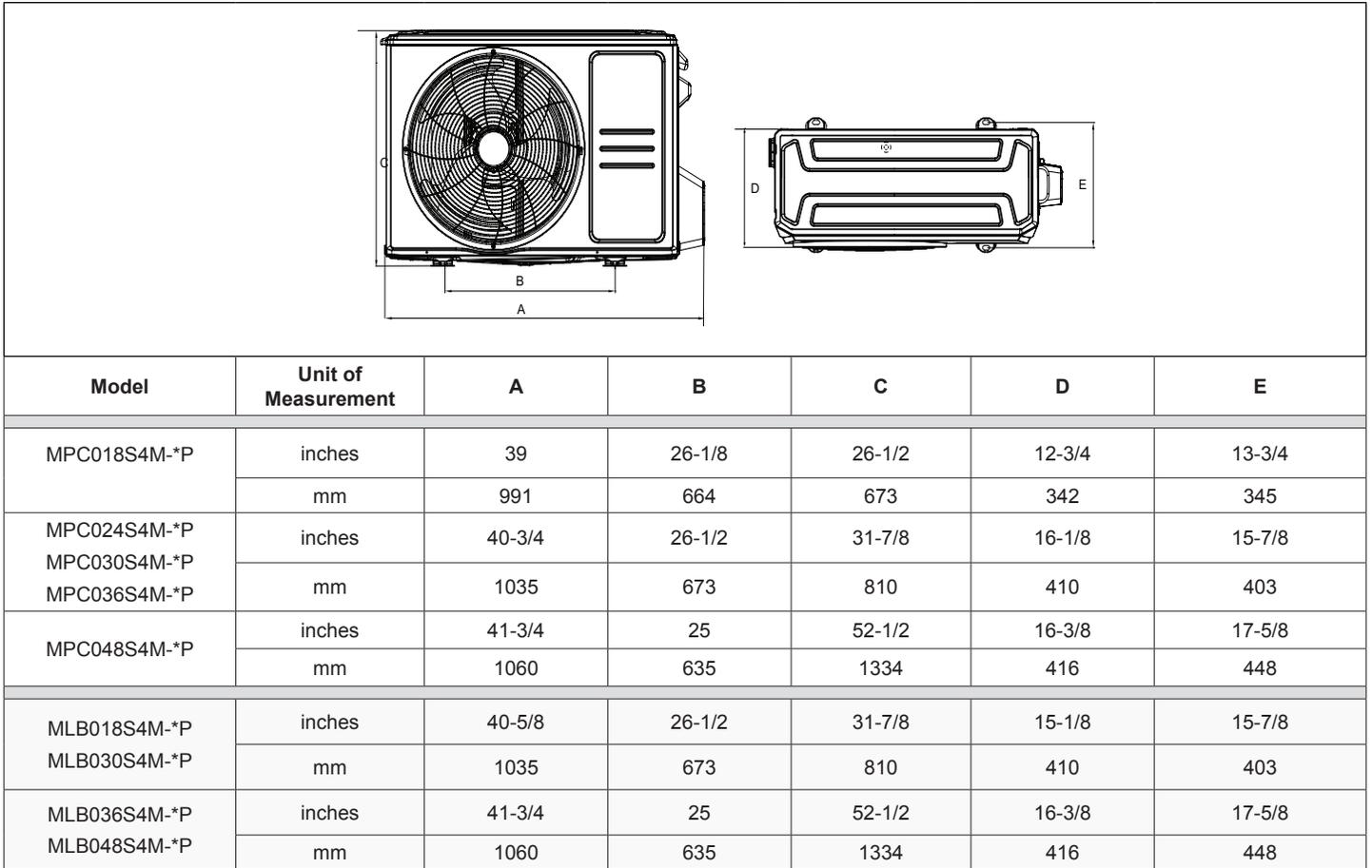
**Figure 28. Multi-Zone Outdoor Unit Dimensions - Inches (mm)**
