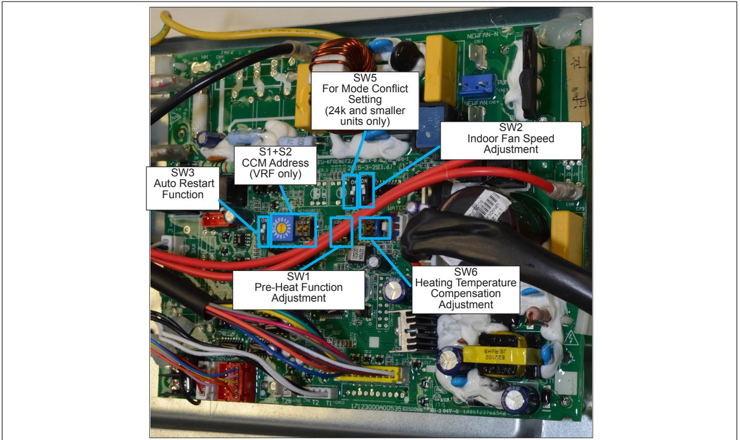
Figure 12. MWMC and 3WMC Main Control Switches
