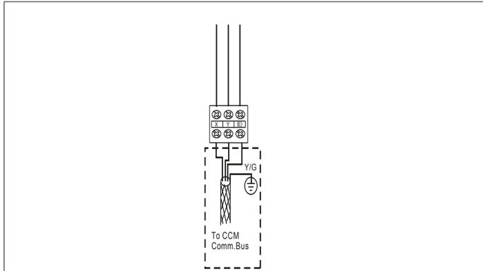
Figure 23. Typical Central Controller Connection Point Example
