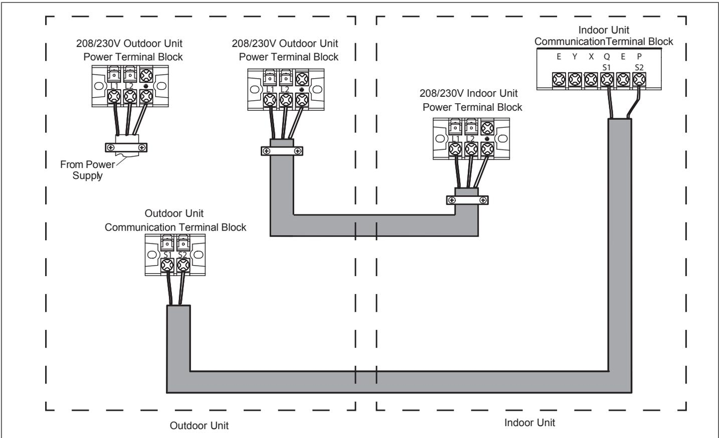
**Figure 20. Communication - Single-Zone Wiring 36K and 48K Only**
