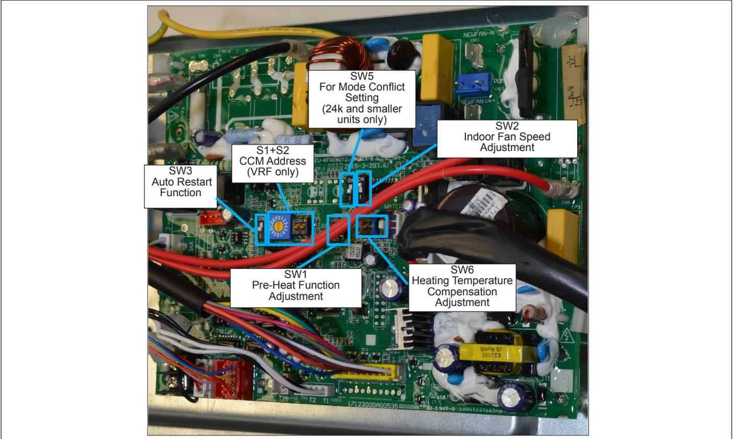
Figure 14. MCFA and MCFB Main Control Switches
