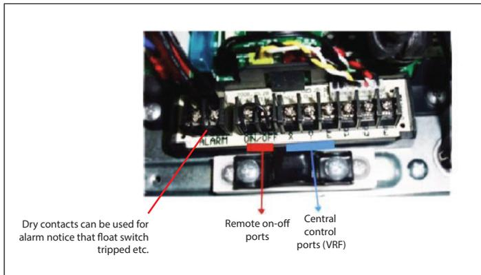
Figure 25. Indoor Unit Connection Points for ON/OFF
