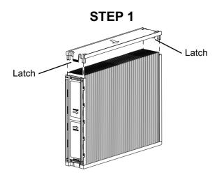
Remove the top/bottom panel by pressing inward on both latches and pulling upward.
