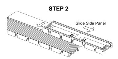
Collapse the filter media. Slide each side panel off of the filter media.
