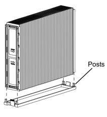
Place the top/bottom panel on a flat surface with posts pointing upward. Expand filter media. Position side panels over the posts and snap into place.
