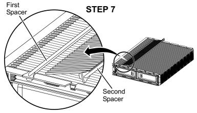
Slide the second spacer into the pleats directly behind the first spacer. Pull the inserted spacer into the next slot and snap it into place. Continue with the remaining spacers.
