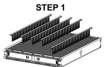
Grasp both ends of each spacer and pull up to remove.
