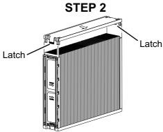
Remove the top/bottom panel by pressing inward on both latches and pulling the panel upwards.
