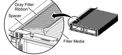
Place the first spacer onto the gray filter ribbon and hold the spacer at a 30 degree angle. When the spacer is positioned properly, carefully slide it down into the pleats and snap it into place.
