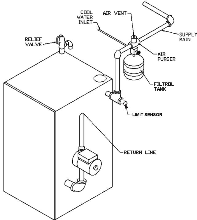
Figure 5 - Chilled Water Piping
