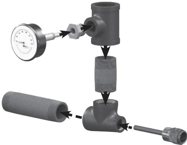
Verify clean water supply is available to water inlet valve. Install sand strainer when water supply is from a well or pump.
