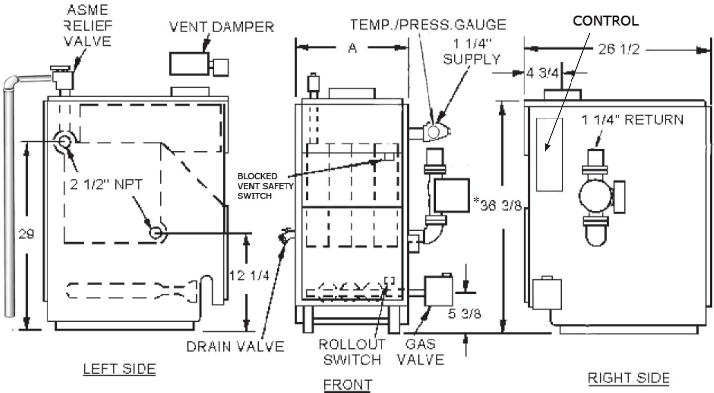
\* Minimum acceptable height for low water cutoff probe.
