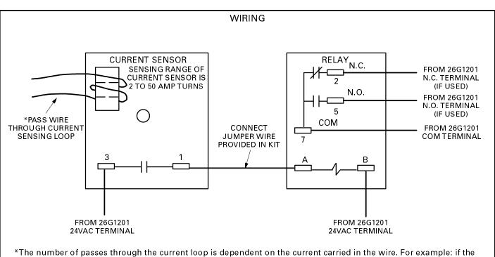
wire carries a minimum of 2 amps, one pass through the current loop is sufficient. If wire carries a minimum of 1 amp, two passes through the current loop is required. (One amp, multiplied by two passes, equals two amp turns.)
