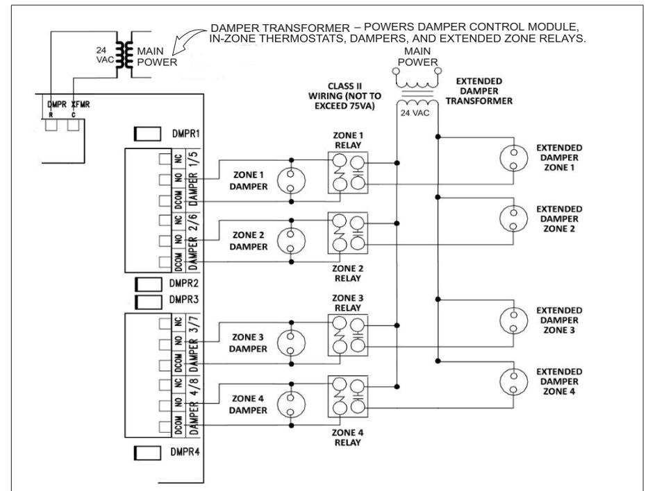
**Figure 4. Damper and Extended Damper Wiring Diagram**
