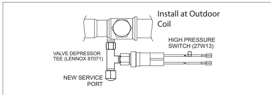
**Figure 5. Tee and Vapor Line High Pressure Switch**
