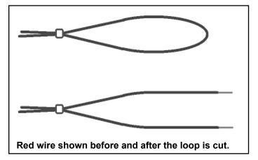
Wire nut one wire from the float switch to one of the red wires as seen below. Do the same for the second float switch wire. It is recommended the wire nut connections be sealed with electrical tape to minimize exposure to moisture.
