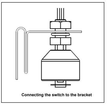
Once the switch has been seccurely fastened to the bracket, the assembly can be mounted to the end of the drain pan as seen below. Be sure to push the bracket down onto the pan as far as possible to ensure more accurate function of the switch.
