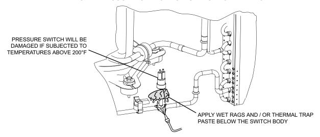
TO PREVENT DAMAGE TO PRESSURE SWITCH PLASTIC COMPONENTS, WET RAGS AND / OR THERMAL TRAP PASTE MUST BE APPLIED BELOW THE SWITCH BODY BEFORE BRAZING. WET RAGS MUST BE LEFT ON PROTECTED AREA UNTIL BRAZED JOINT HAS COOLED DOWN TO AMBIENT TEMPERATURE TO PREVENT MIGRATION OF HEAT INTO THE SWITCH BODY.
