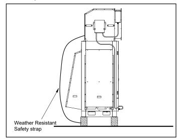
Figure 6. Secure Unit with Safety Strap (Back)
