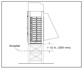
Figure 4. Elevate Unit Above Snow Level
