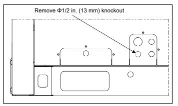
Figure 12. Remove Knockout
