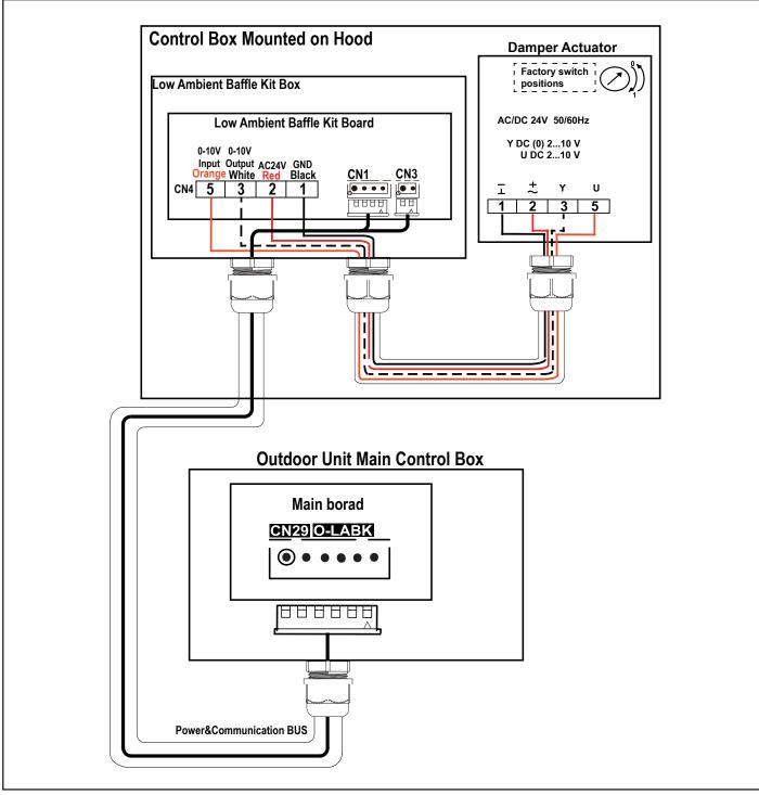
Figure 16. Connection Diagram
