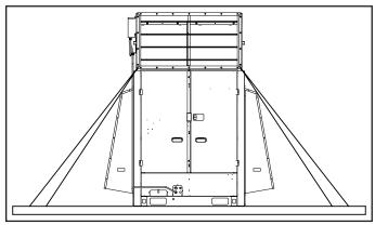
Figure 7. Secure Unit with Safety Strap (Sides)
