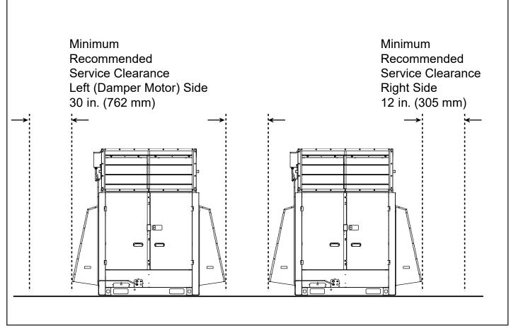
Figure 3. Distance Between Units with Kit Installed
