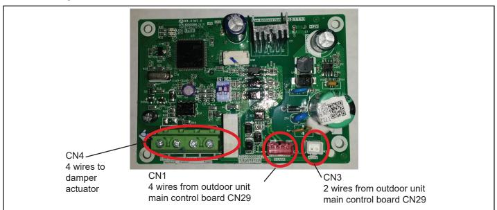
Figure 13. Damper Motor Control Board
