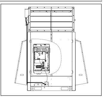
Figure 14. Outdoor Unit Control Board Location
