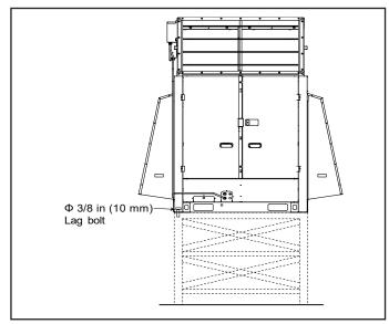
Figure 5. Secure Unit to Weather Resistant Support
