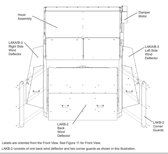
Figure 9. Attach Corner Panels LAKB Only Using Provided Screws
