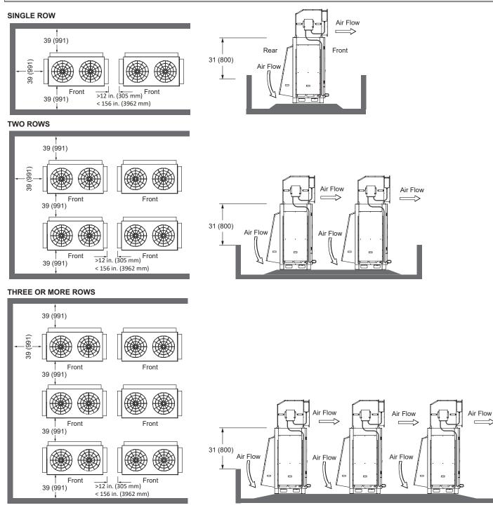
**NOTEs -** Discharge air duct will remain free of obstructions at a minimum distance of 18 ft. (5.5 m). Discharge air shall not be directed toward operable windows or building fresh air intakes.
