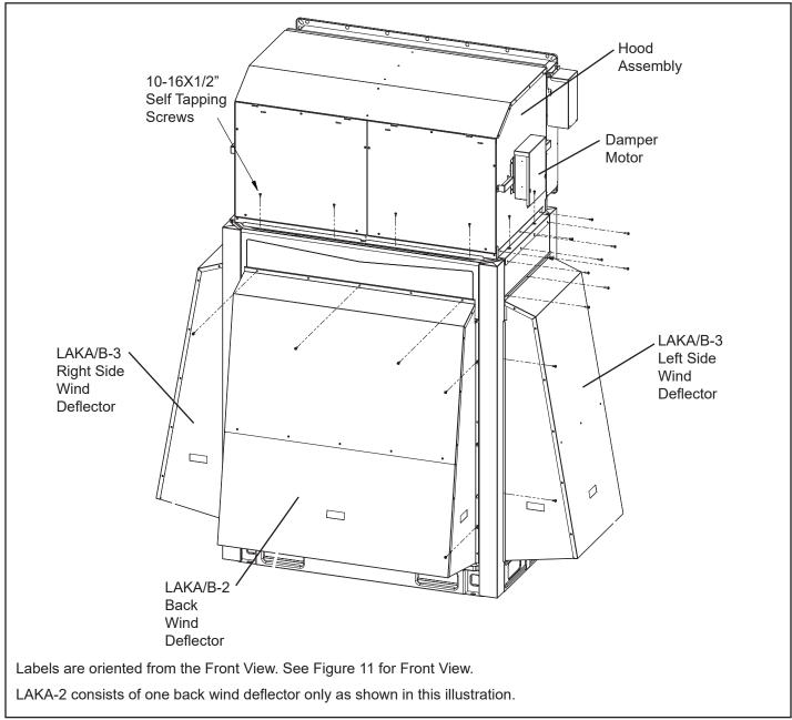
Figure 8. Attach Hood and Wind Deflectors Using Provided Screws
