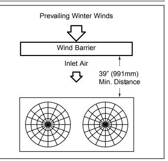
Figure 1. Prevailing Winds Barrier
