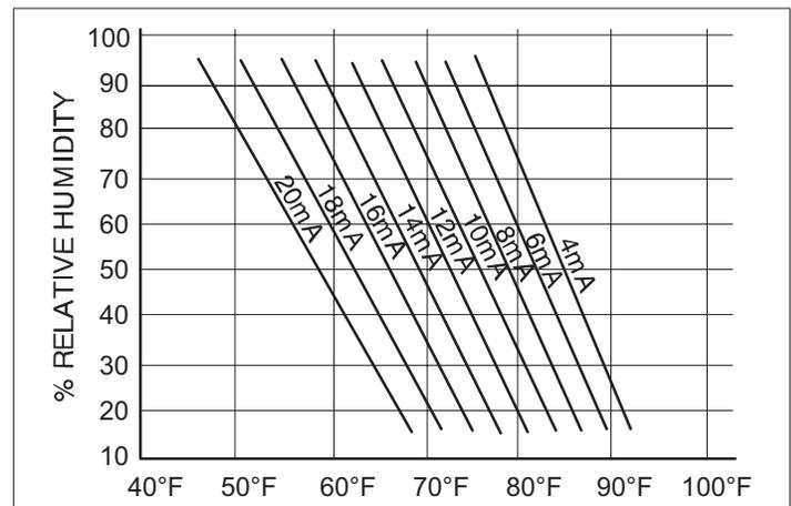
**Figure 31. Enthalpy Sensor Output Current Honeywell C7400**
