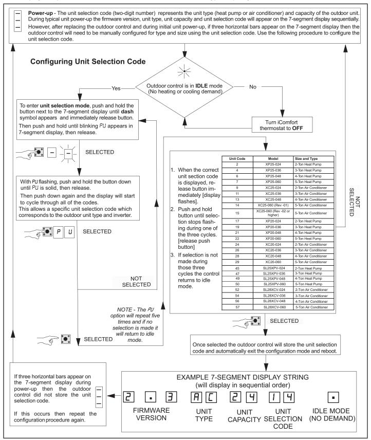
FIGURE 1. Configuring Unit Selection Code
