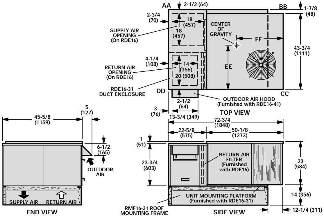
**CHA16H-261 WITH REMD16-41 ECONOMIZER, RDE16-31 DUCT ENCLOSURE AND RMF16-31 ROOF MOUNTING FRAME**
