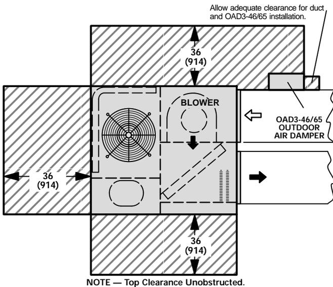
**CHA16H-261 UNIT WITH RDE16-31 DUCT ENCLOSURE AND REMD16-41 ECONOMIZER DAMPER SECTION**
