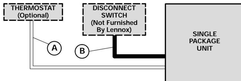
A — \*Four Wire 24V (Electro-mechanical)
