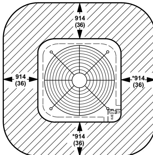
NOTE—1219 mm (48 in.) clearance required on top of unit.
