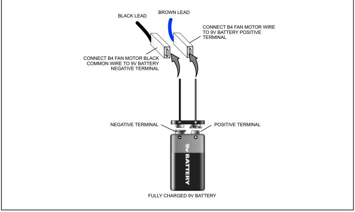
Figure 46. VDC Voltage Check
