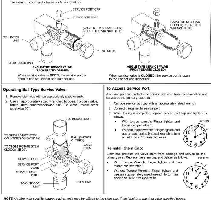
Figure 3. Angle and Ball-Type Service Valves
