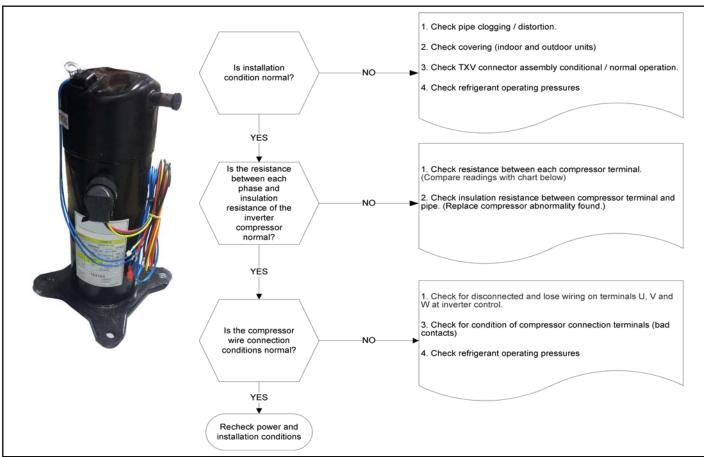
Figure 34. Compressor Operation, Checkout and Status/Error Codes
