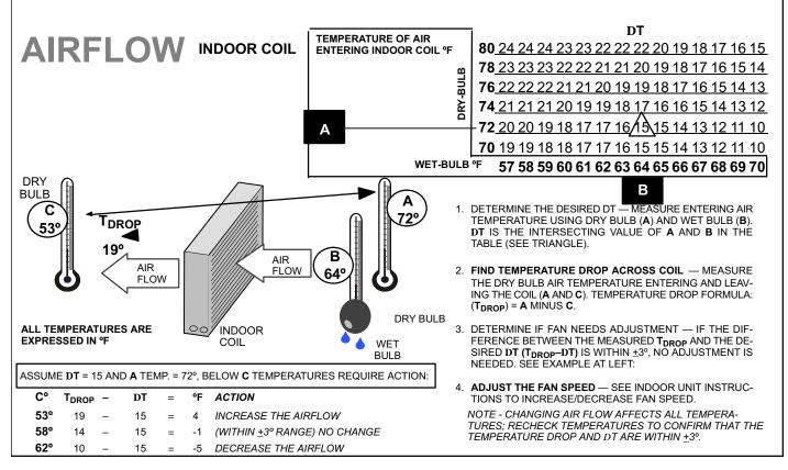
Figure 55. Checking Indoor Airflow over Evaporator Coil using Delta-T Chart
