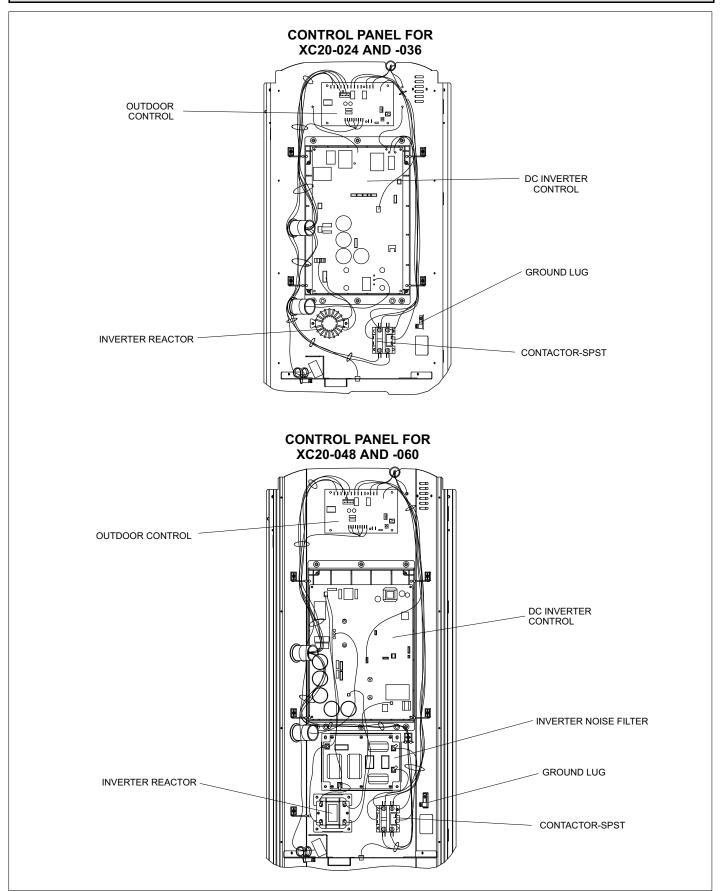
Figure 1. Control Panel Components
