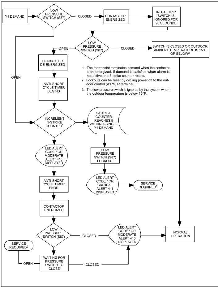
Figure 28. Low Pressure Switch (S87) Sequence of Operation (All Versions)
