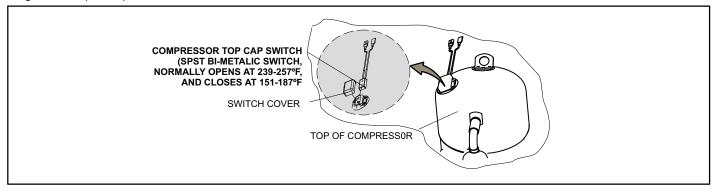
Figure 40. Top Cap Thermal Sensor Switch
