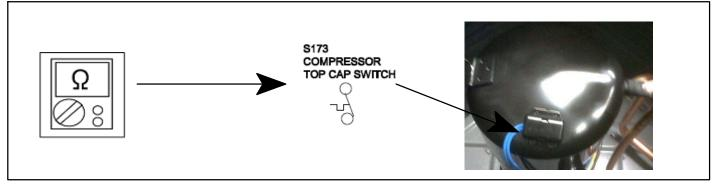
Figure 41. Verifying Top Cap Thermal Sensor Switch
