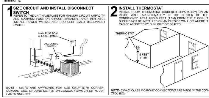
Figure 12. Electrical Installation
