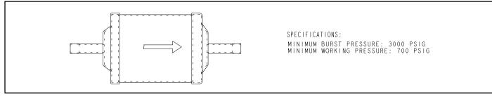
Figure 39. Liquid Line Filter Drier
