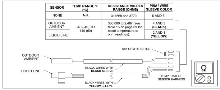
Figure 49. Temperature Sensor Specifications
