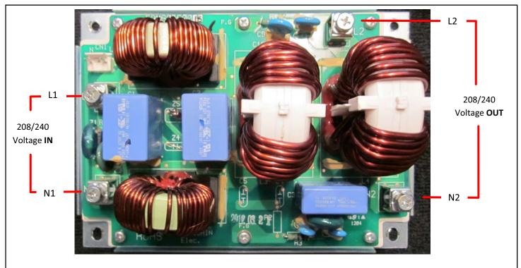
Figure 44. XC20 4- and 5-ton filter board (EMC)
