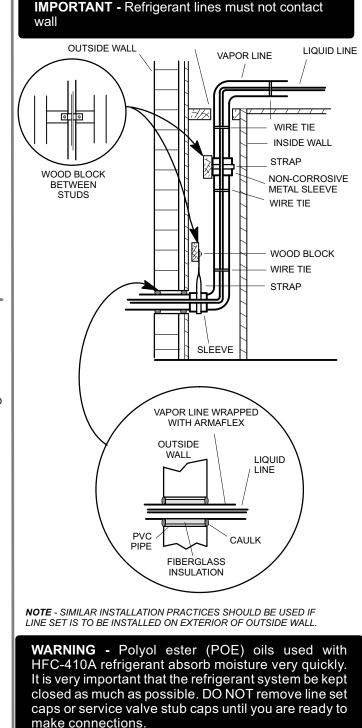
Figure 7. Line Set Installation
