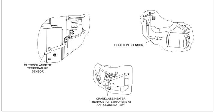
Figure 50. Temperature Sensor Locations
