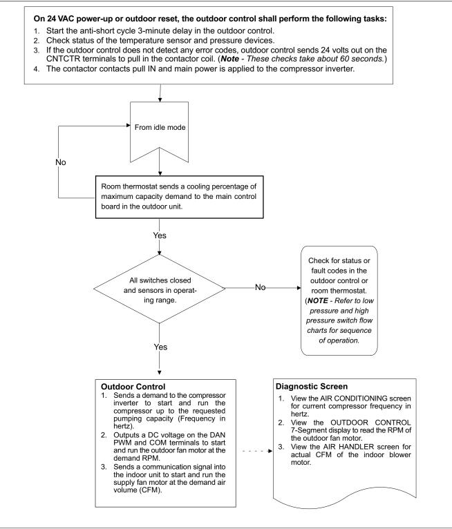
Figure 27. 24 Volt Power-Up or Outdoor Reset
