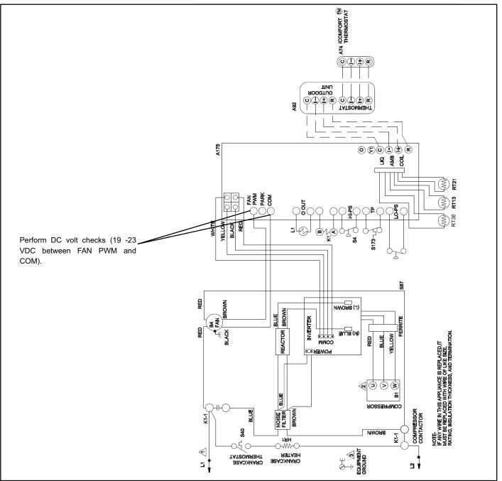
Figure 45. VAC Voltage Check
