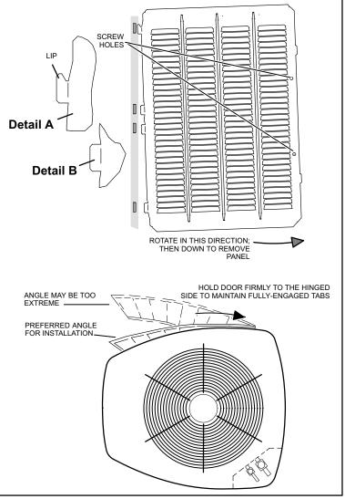
Figure 6. Removing and Installing Panels
