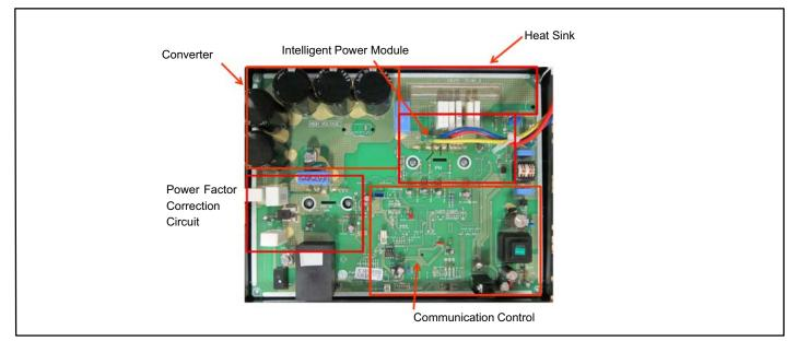
Figure 52. 4- and 5-Ton Unit Inverter
