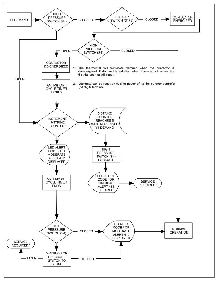
Figure 32. High Pressure Switch (S4) Sequence of Operation (All Versions)
