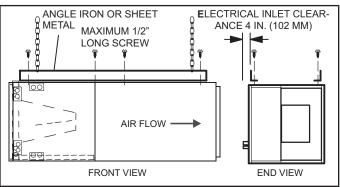
FIGURE 14. Suspend Horizontal Unit
