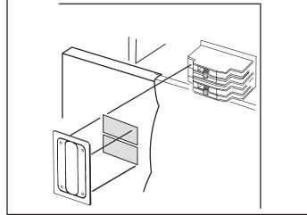
FIGURE 12. Typical Circuit Breaker Cover Installation
