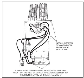
FIGURE 7. Installing the Heat Element Assembly
