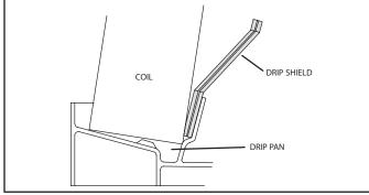
FIGURE 20. Downflow Drip Shields
