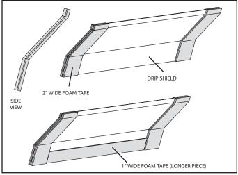
FIGURE 19. Applying Foam Tape to Drip Shield
