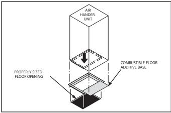
FIGURE 21. Downflow Combustible Flooring Base
