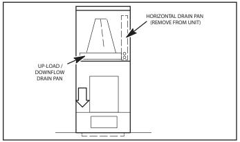
FIGURE 18. Downflow Discharge Position
