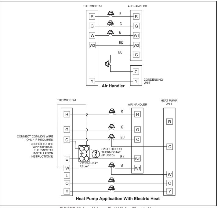
FIGURE 27. Low Voltage Field Wiring Electric Heat
