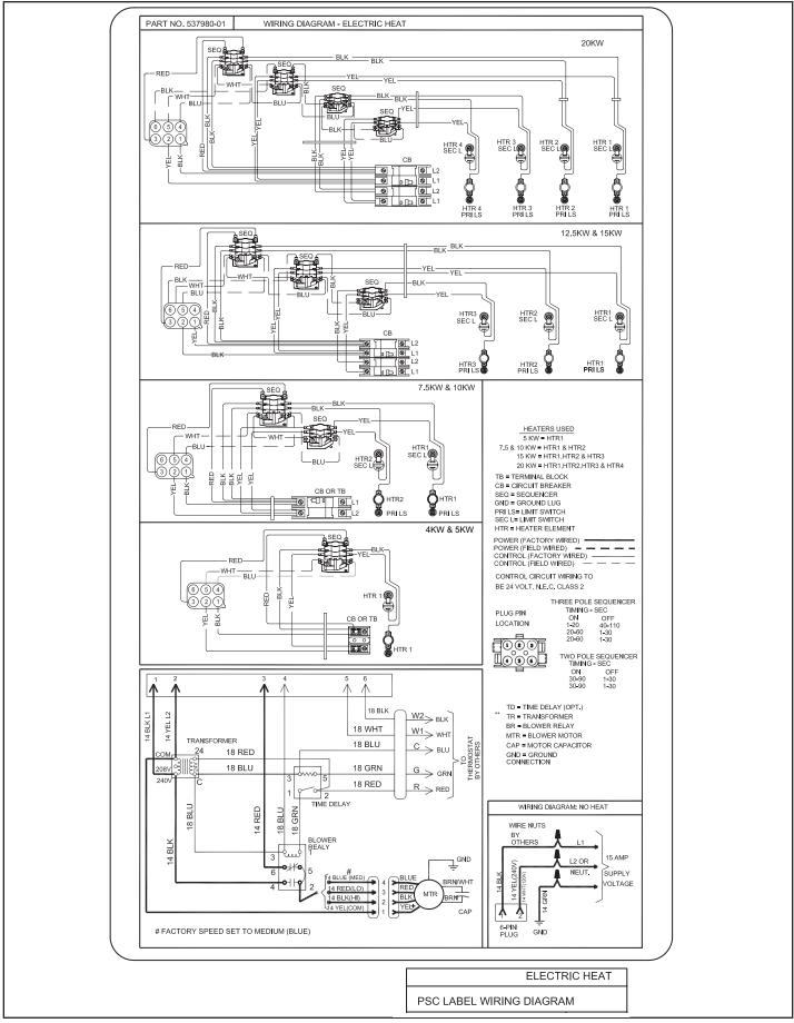
FIGURE 28. Unit Wiring Diagram – Electric Heat and Air Handler
