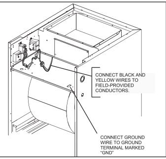
FIGURE 25. Making Electrical Connections
