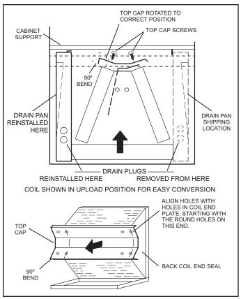
FIGURE 14. Field Modification for Left-Hand Discharge
