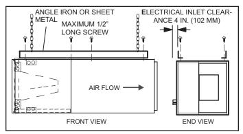
FIGURE 13. Suspend Horizontal Unit
