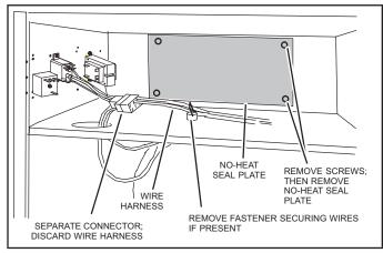
FIGURE 5. Prepare to Install Heat Element
