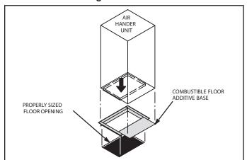
FIGURE 18. Downflow Combustible Flooring Base
