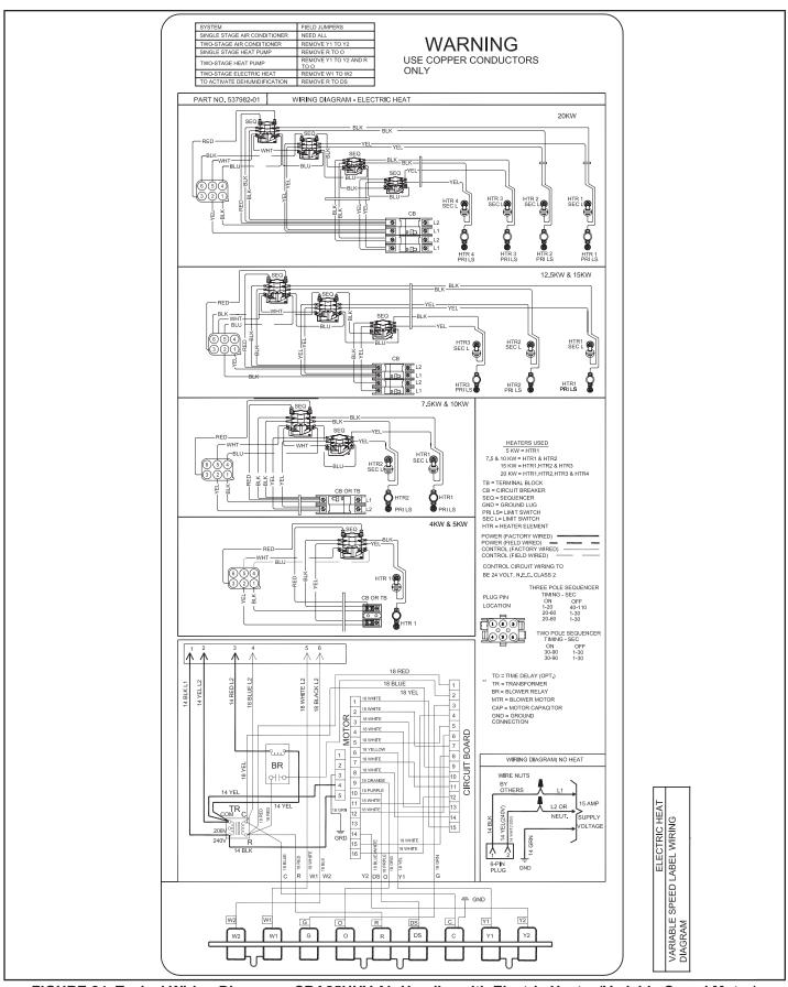
FIGURE 24. Typical Wiring Diagram – CBA25UHV Air Handler with Electric Heat – (Variable-Speed Motor)
