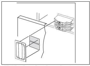
FIGURE 11. Typical Circuit Breaker Cover Installation
