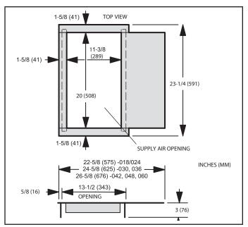
FIGURE 19. Downflow Combustible Base Dimensions
