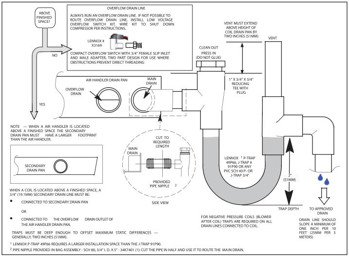
FIGURE 21. Typical Main and Overflow Drain Installations
