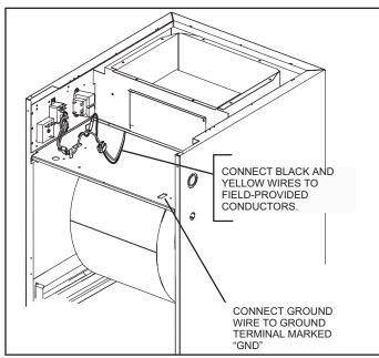
FIGURE 23. Making Electrical Connections 208 VOLT CONVERSION
