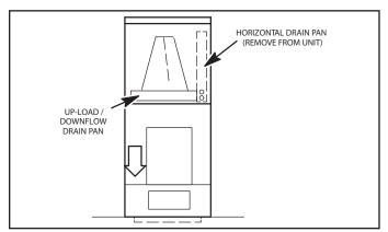
FIGURE 17. Downflow Discharge Position
