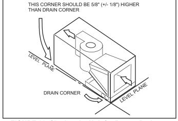
FIGURE 22. Sloping the Unit for Proper Drainage
