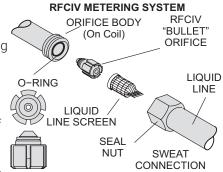
• Equalizes pressure shortly after compressor stops, unit starts unloaded, eliminating need for additional controls
