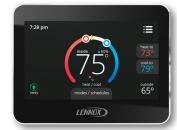
Offers enhanced capabilities including humidification / dehumidification / dewpoint measurement and control, *Humiditrol*® control, and equipment maintenance reminders.
