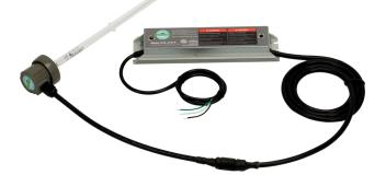
Germicidal lamp emits C-Band ultra-violet (UVC) energy at 253.7 nanometers, which is proven to be effective in reducing microbes such as viruses, bacteria, yeasts, and molds. This process either destroys the organism or controls its ability to reproduce. UVC germicidal light greatly reduces the growth and proliferation of mold and other bioaerosols (bacteria and viruses) on illuminated surfaces (particularly coil and drain pan). Surfaces must be cleaned prior to UVC light being installed.
