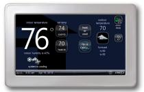
recognizes model and serial number information for iComfort<sup>®</sup> Communicating products to simplify system setup.
